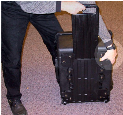
Figure 1-1. Use the release catch to operate the handle on the Pelican case
