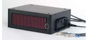
The 'Desert Proven' Filter system is also included keeping fine particle filth out of the disk and power systems. External MiniSAS 4 channel cables, providing an amazing 2.4GB/Sec.
